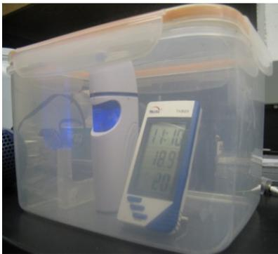
Figure 17: Humidity chamber with the LPG fiber sensor fixed on a plastic frame, the moisture generator, and the humidity-meter.
