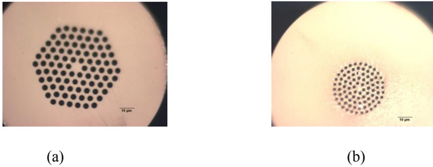
Figure 1. Cross-sectional optical micrographs of endlessly single-mode Index Guide-Photonic Crystal Fibers (IG-PCFs) (fabricated by Yangtze Optical Fiber and Cable Company Ltd.) with (a) 5 rings of air-channel round latticed in cladding and (b) 5 rings of air-channel hexagonal latticed in cladding section with a perfect electric and magnetic conductor boundary condition applied along symmetrical planes.
